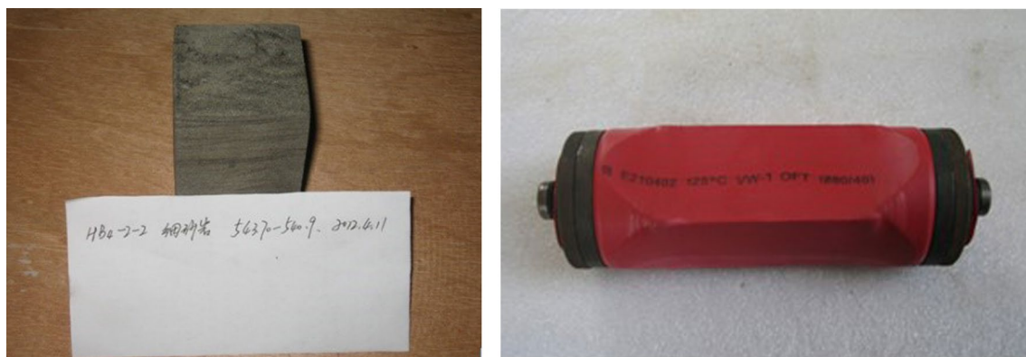
Fig. 1 Standard prepared specimen (left) and post-packaged specimen (right)
